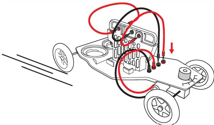
Note: After long time running, the car speed will slow or stop. If you want to continue to run the car, you should pull out the anode metal plate to clean it up with the running water. Replenish some salt solution to the fuel cell tank. Place back the anode metal plate to the cathode fuel cell tank, the car will continue to run. After use, you should pull out the anode metal plate and clean up the fuel cell tank with the running water. Keep them dry for storage.
