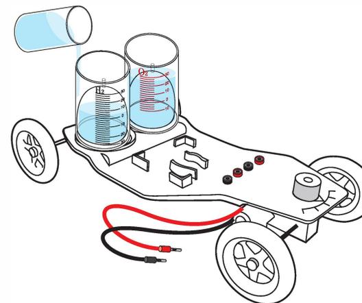
g. Fit the reversible fuel cell onto the car frame, just in front of the containers and make sure the red plug is located on the O<sub>2</sub> container side.
