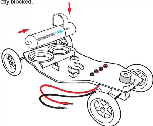
e. Connect the other end of the pressure regulator tube to the fuel cell higher nozzle (close to the red plug). Then lightly screw the pressure regulator to the HYDROSTIK PRO. Stop to screw as soon as both parts fit together.
