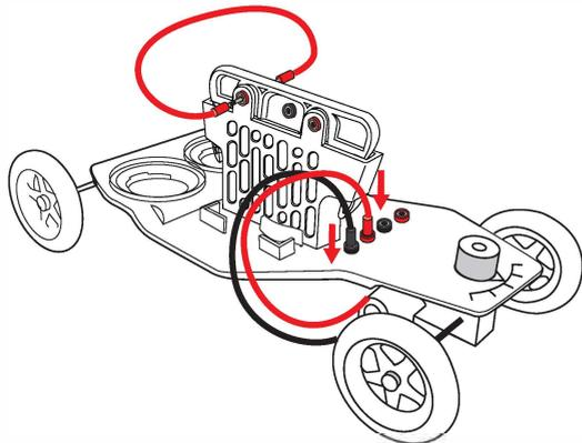
d. Connect the black long wire in the central plug and the red on in the front red plug. Connect the other end of these wires into the car right plugs. The car starts to move. Ensure that you have connected the wires in the good sense. On the contrary, the car will go back.
