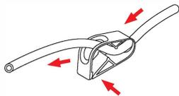
b. Unscrew the bolt on the pressure regulator, and put it around the tube. Connect the end of the tube to the pressure regulator. Ensure the connection is tight, and then screw the bolt to the pressure regulator.
