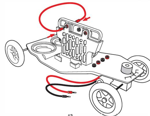
c. Connect the car engine wires to the plugs on the car.
