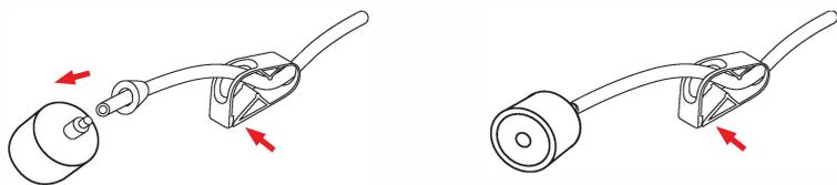
c. Put the purging valve on the 5 cm long tube and ensure the connection is tight. Then, connect it to the nozzle you can see on bottom of the mini fuel cell.
