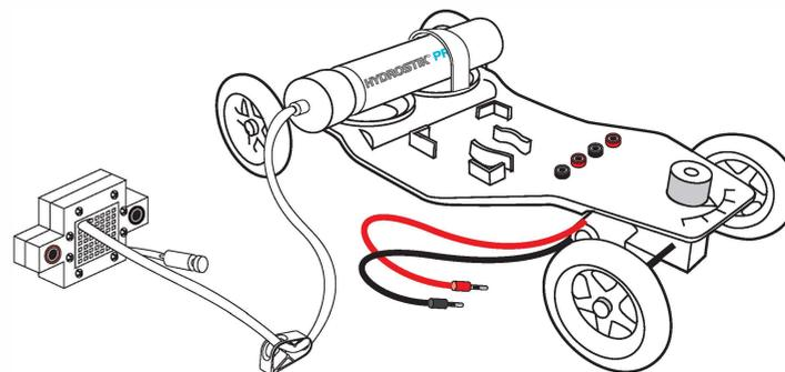
f. After this place the mini fuel cell on the slot located on the car frame top. Ensure they fit well.
