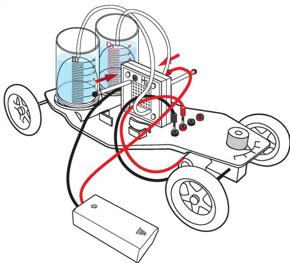
c. Then, connect the engine wires which exceed the bottom of the car, to the closest red and black plugs.
