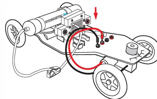
h. Connect the two wires to the red and black plugs on the car frame. Connect the other end to the fuel cell.
